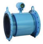
Magnetic bi-directional flowmeter with stainless steel electrodes, 4-20 mA output, local display, NEMA 4X housing, and no moving parts to wear out
