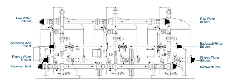
H&T "Plug & Play" Water Filtration Systems feature a versatile "Daisy-Chain" design that allows for coupling one to three vessels.
