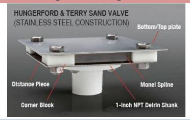
The "Self-Cleaning" Sandvalve underdrain nozzles from H&T feature patented free-floating splines around the periphery of each nozzle device. The free-floating splines which are constructed of durable Monel steel float freely between a guided path defined within the corner blocks in a manner similar to that of a sliding door through tracks.
